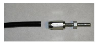
Step #3 – While holding the hose firmly in one hand, begin threading the Field Install Nut/Stud assembly counterclockwise onto the O.D. of the hose. Continue threading the Field Install Nut/Stud onto the hose until you can no longer turn it by hand.
